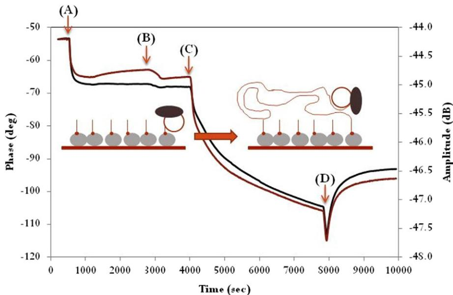
**Fig. 5.** Real-Time plot of RCA on-chip at RT (red line: amplitude; black line: phase). (A) Surface saturation with neutravidin. (B) Binding of a biotinylated primer to neutravidin. (C) Loading of the RCA mix (circular padlock, phi29 polymerase etc.) on the sensors surface – incubation for 60 min in static mode. (D) Buffer rinsing under flow. Inset: Schematic depiction of the device surface during on-chip RCA amplification and detection.
