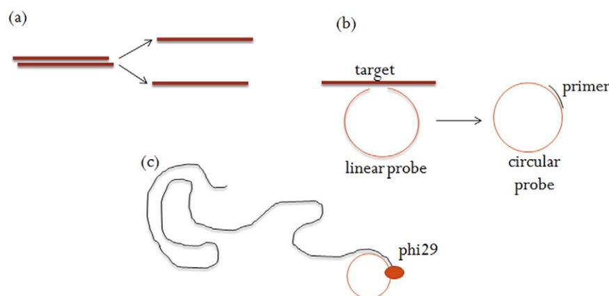
**Fig. 1.** Schematic depiction of the RCA method: (a) DNA target denaturation, (b) padlock hybridization to DNA target and circularization; primer hybridization and (c) primer elongation and DNA amplification with phi29 polymerase.
