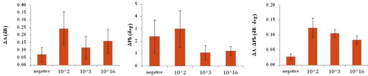
**Fig. 4.** Acoustic detection results for RCA products prepared off-chip at 30 °C using from 100 up to  $10^{16}$  DNA target copies. The three charts display the measured values related to changes in the amplitude (dB), phase (deg) and calculated acoustic ratio (dB/deg).
