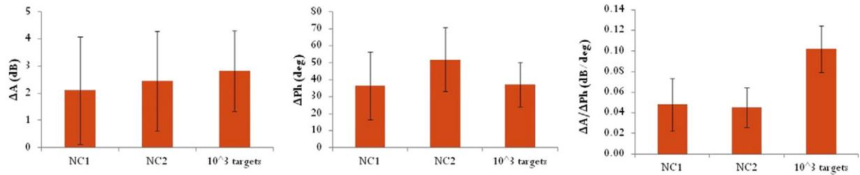
**Fig. 6.** Acoustic ratio average values and standard deviations for experiments where RCA was conducted on-chip. Negative control 1 (NC1) represents reactions with no circular probes, whereas negative control 2 (NC2) represents reactions where the probes were present but there was no complementarity with the immobilized primers for initializing the RCA. Positive samples represent RCA reactions with 1000 copies of chemically synthesized target as a starting template.
