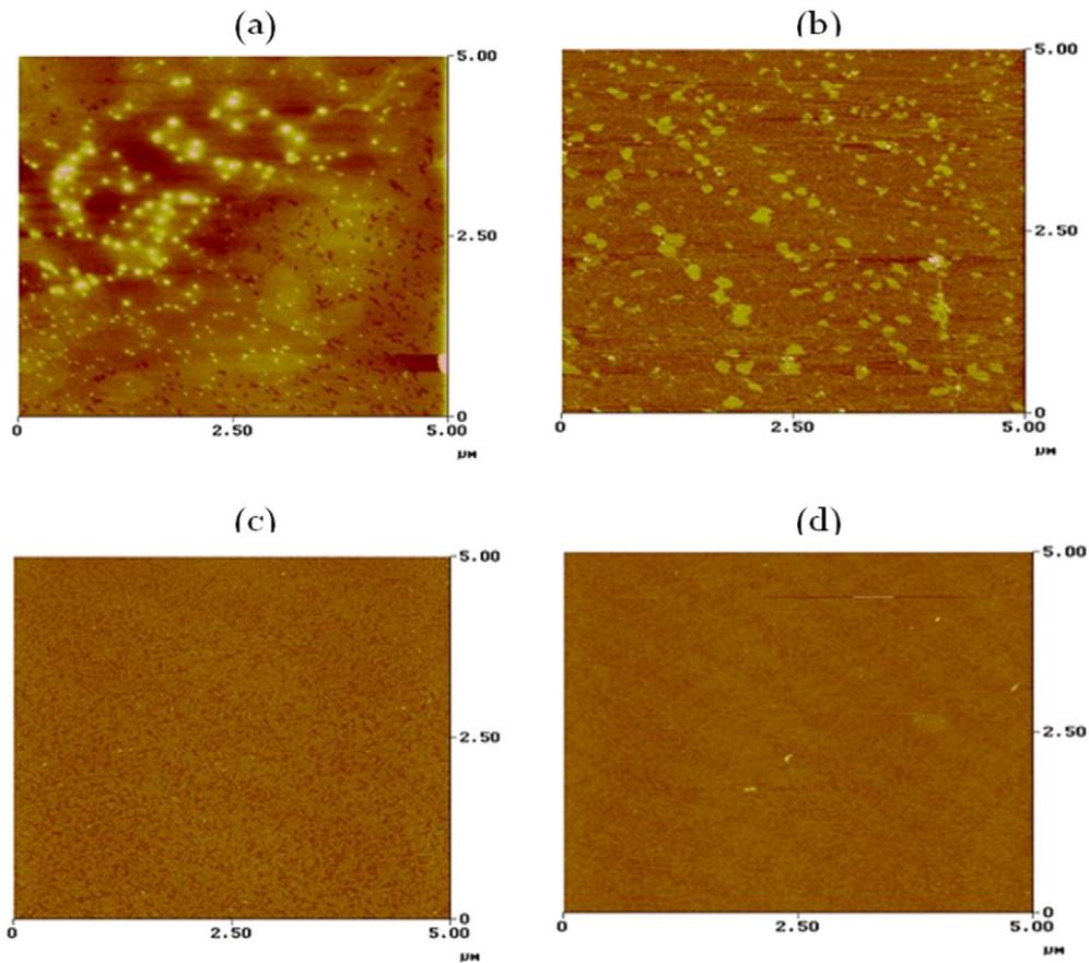
**Fig. 2.** AFM images of RCA products upon amplification of an initial template of  $10^{16}$  DNA targets before (a) and after (b) purification; and the negative sample (without DNA targets) before (c) and after (d) purification.
