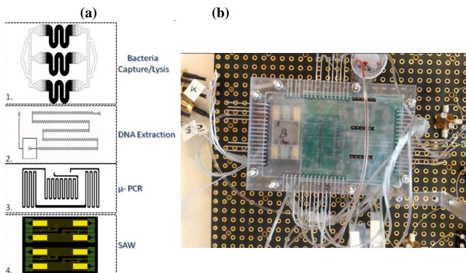
**Figure 2.** (a) The individual modules of the LOC cartridge comprise the following modules 1. cell capture and lysis; 2. DNA extraction (purification); 3.  $\mu$ PCR; and, 4. acoustic bochip. (b) Picture of the assembled LoC prototype with the integrated modules.
